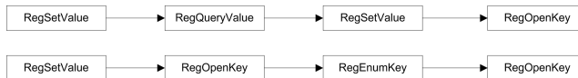
Figure 3: API call sequences present in malware traces and absent in benign traces
